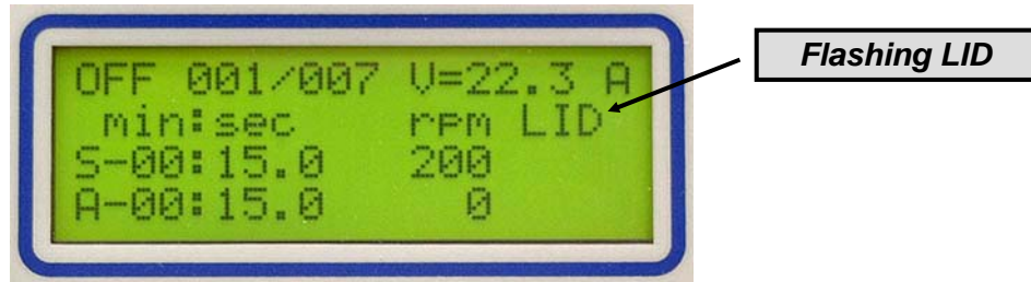
Figure 3-2 FLASHING LID DISPLAY
